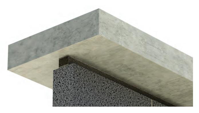
A versatile, compressible intumescent sealing strip for joints in compartment walls and floors. The AIM intumescent expansion joint is a high quality composite sandwich of fire retardant foam and intumescent seals. This product is held in place by compression, without the need for mastics or adhesives.
